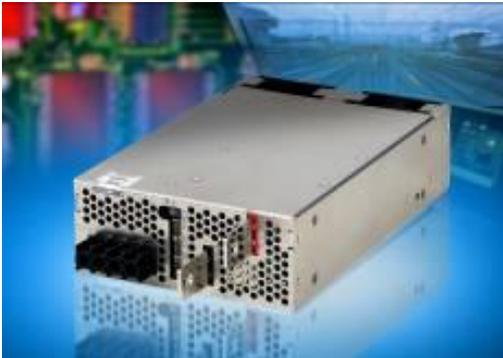
*Fig. 3: This unit, a SWS1000L series power supply, delivers up to 1 kW of output power and features alarm signals and active current sharing. Two or more can be connected in parallel with external isolation diodes to form a redundant and fault tolerant power system.*
