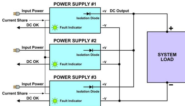
Fig 1: In this typical redundant power system, three power supplies interface in parallel to the system load via internal ORing diodes.
