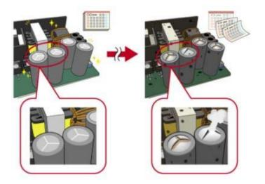
The <u>countermeasure</u> is during the system design, to ensure that there is sufficient distance around the power supply to allow free air to circulate. If a fan is being used to cool the product, the airflow should be directed across the power supply as detailed in the installation manual. Temperature measurements of key components should be performed inside the end system.
