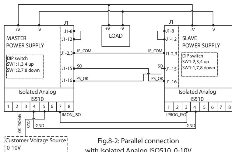
Fig.8-2: Parallel connection with Isolated Analog ISO510, 0-10V
