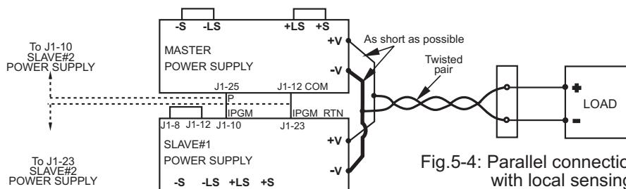
Fig.5-4: Parallel connection with local sensing
