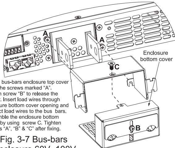
Fig. 3-7 Bus-bars enclosure 60V~100V
