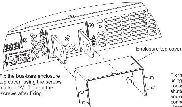
Fig. 3-6 Bus-bars cover 8V to 50V
