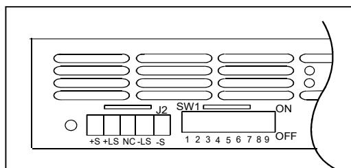
Fig.3-15: Sense connector location
