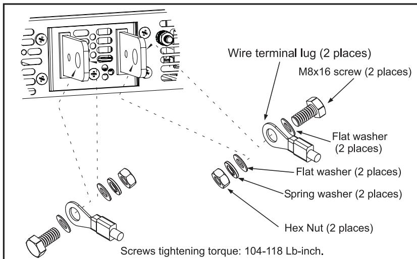
Fig. 3-5: Load wires connection , 8V to 100V models.
