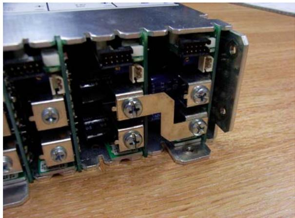
**Example 4 : 2 slot E2 module with voltages combined.**
