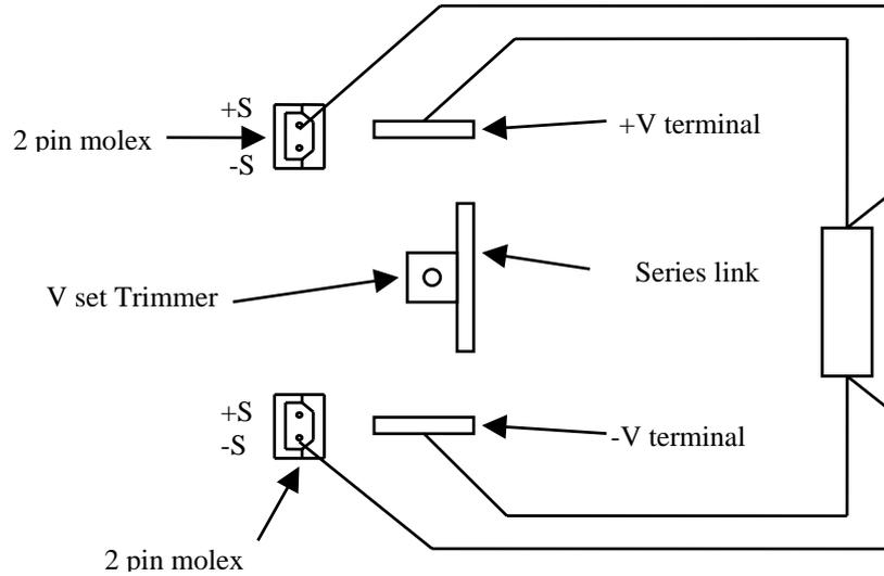
Connect +S from the top 2pin molex connector to +V of the load.
