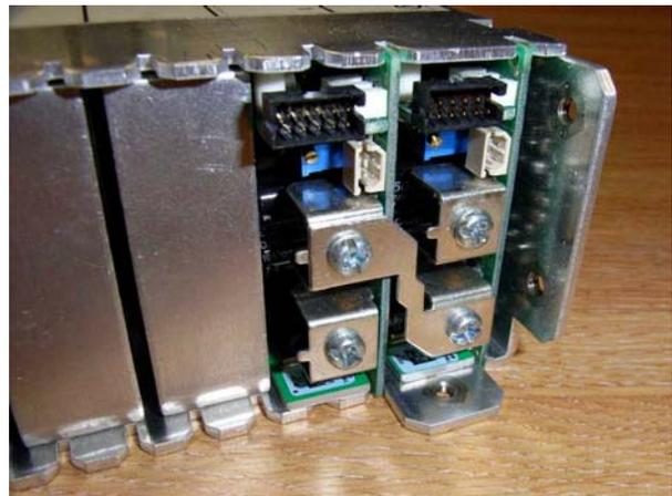
**Example 3 : 1.5 slot D4 module with voltages combined.**
