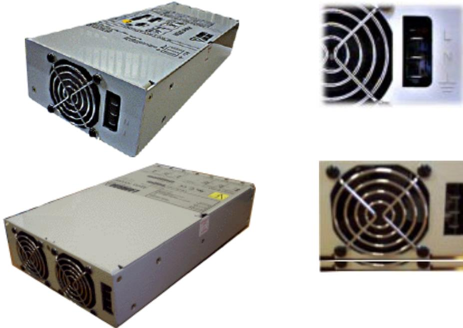
The AC input connection is situated adjacent to the cooling fan inlet as shown above. The 'faston' tabs are tin plated 6.3 x 0.8mm at 9mm centres. Connection is made using insulated 6.35mm 'faston' connectors. Rated at 15amps each.
