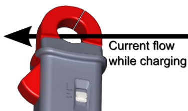
Figure 19: 300A clamp polarity
