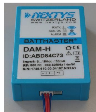
Figure 24: Cable connection to the DAM
