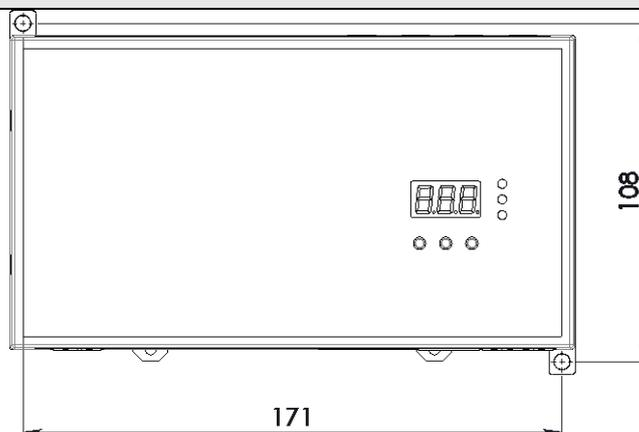
It is possible to install directly on panel or wall using the appropriate fixing points according to the above image.
