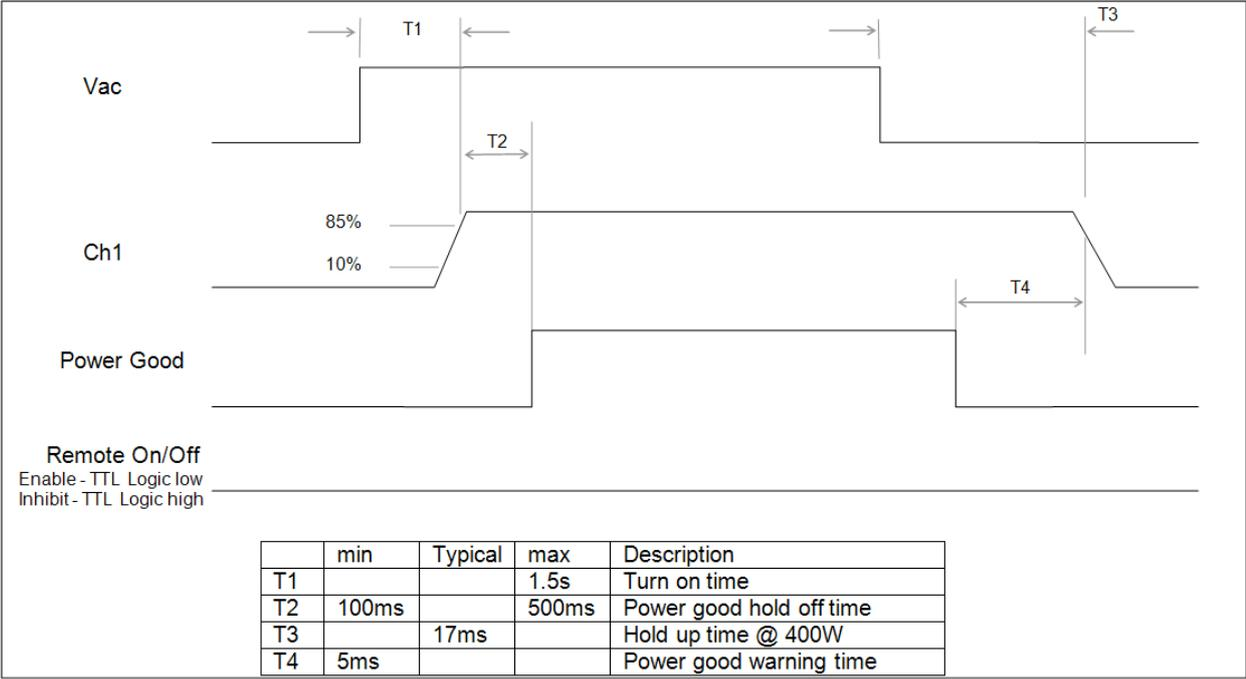
**Figure 4. Output Timing Diagram (Remote ON/OFF Control)**
