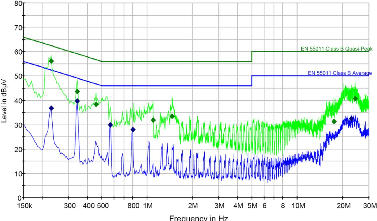
Figure 9. Typical Conducted Emissions result at 400W fan cooled:
