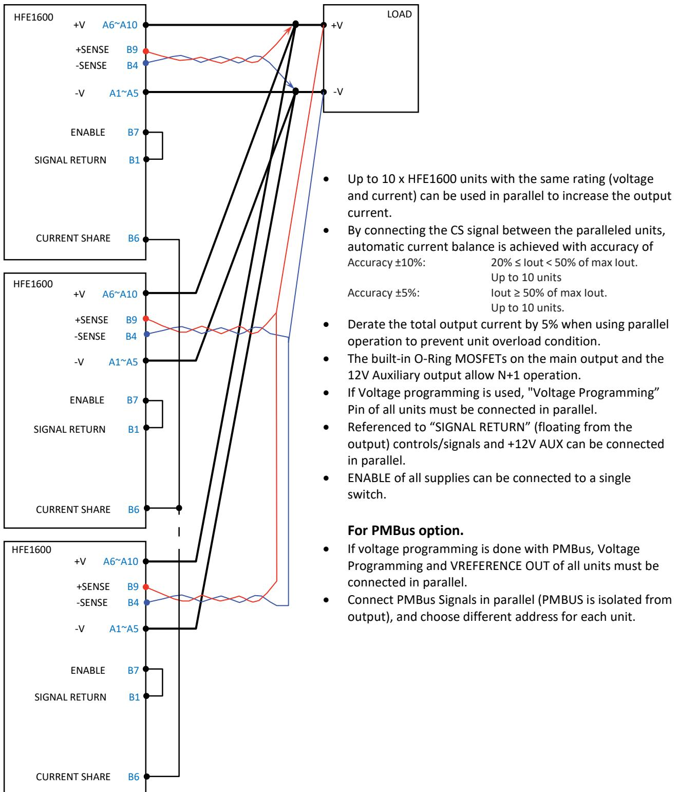
Figure 4–1: Parallel Connection
