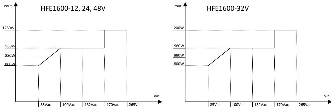
Figure 1-6: Output Power derating at temp 60°C.
