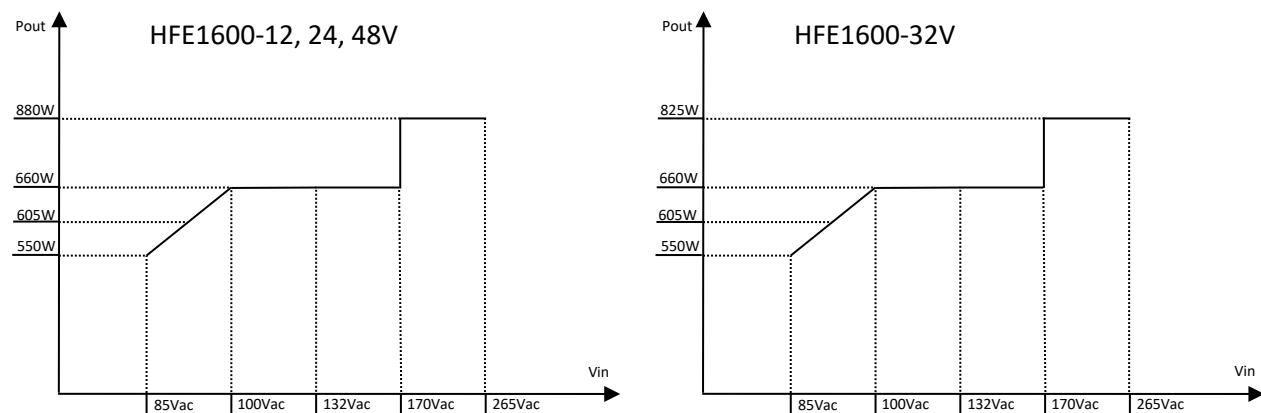
Figure 1-7: Output Power derating at temp 70°C.
