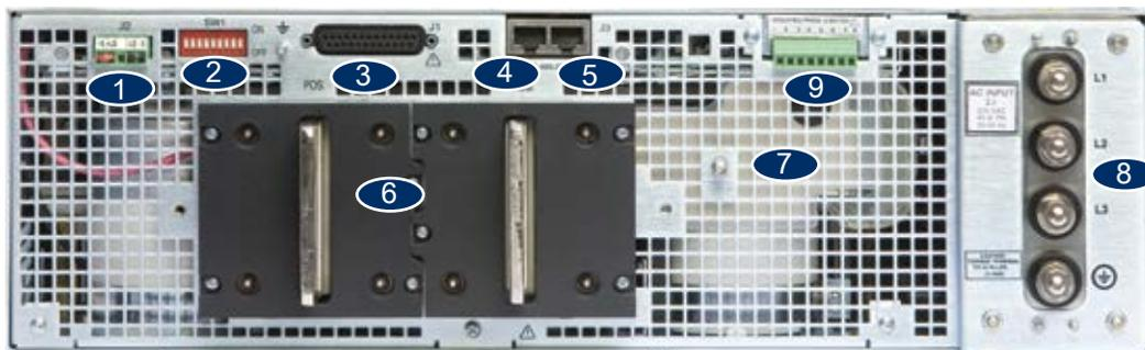
1. Remote/Local Output Voltage Sense Connections.
