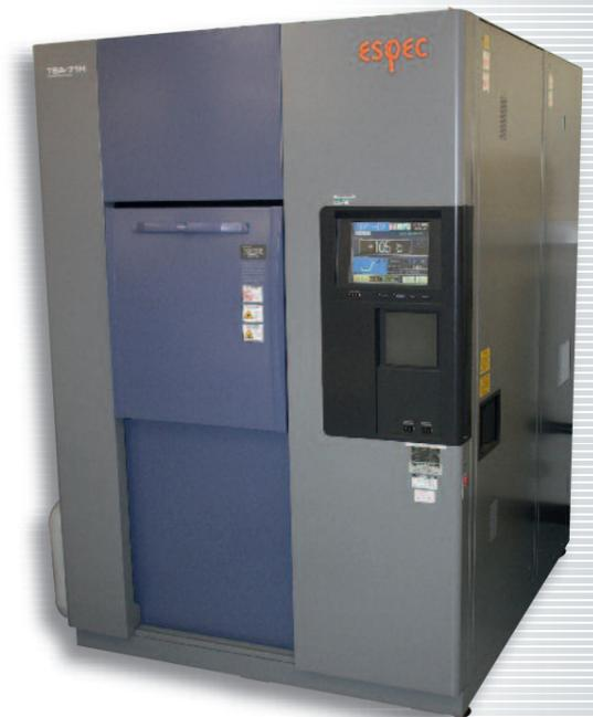
Thermal Shock Test chamber
