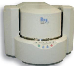
EDX Fluorescence Spectrometer for RoHS evaluation
