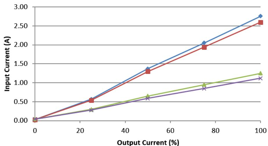
**(4) Input power vs. Output current**
