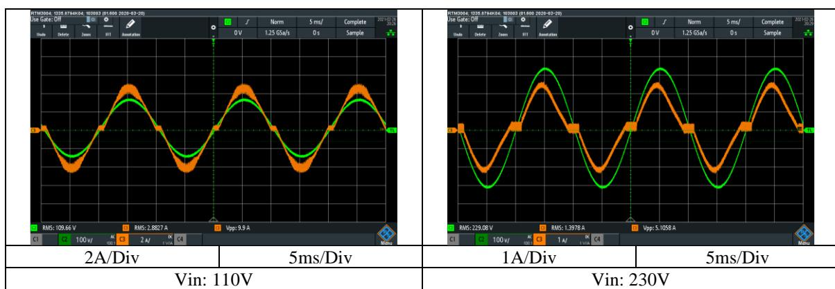
**2.13 Leakage current characteristics**
