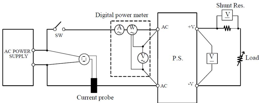
**Circuit 4 used for determination**
