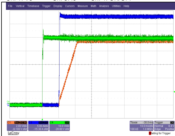
Start-up from Input Voltage Application at Full Load. Ch. 1: Vo Ch. 3: Io Ch. 4: Vin
