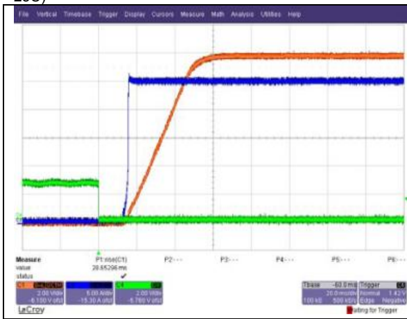
Start-up from on/off Switch at Vin,nom and Full Load. Ch. 1: Vo Ch. 3: Io Ch. 4: ON/OFF
