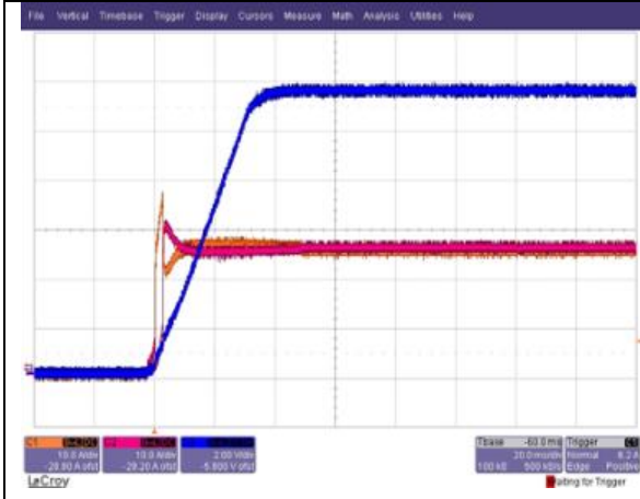
Start-up from on/off switch: 48V in , I o =50A (200% Load) Ch. 1: I o1 Ch. 2: I o2 Ch. 3: V o
