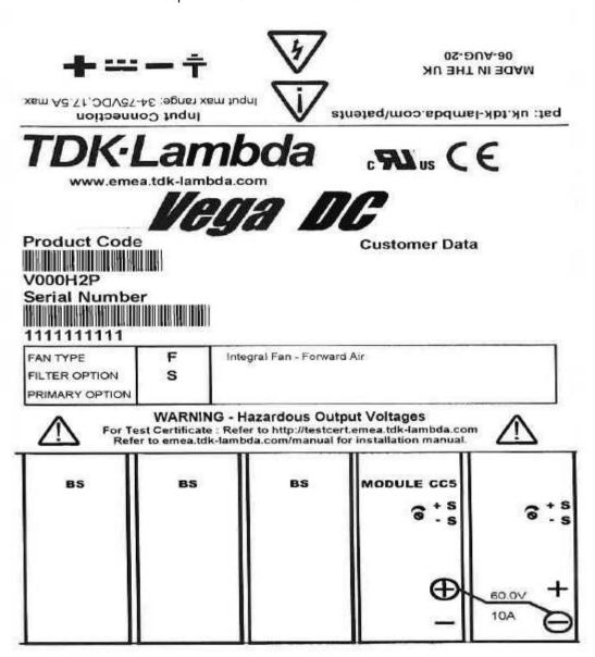
Note: The above markings are the minimum requirements required by the safety lab. For the final production samples, the additional markings which do not give rise to misunderstanding may be added.
