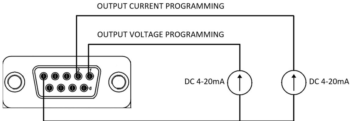
Figure 8–2: Isolated Analog Programming Wiring
