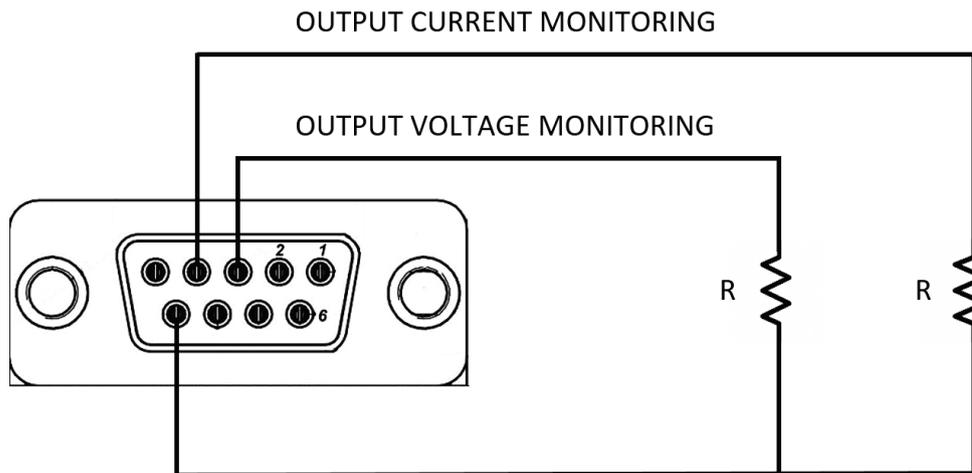
Figure 8–3: Isolated Analog Monitoring Wiring
