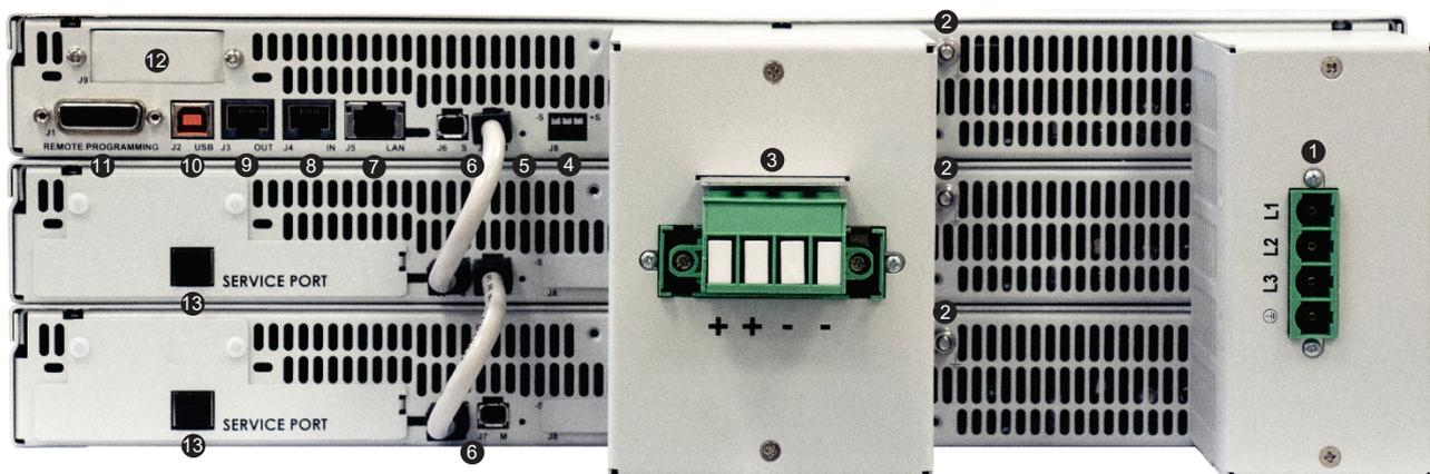
Figure 1-4: Rear Panel Connection and Controls
