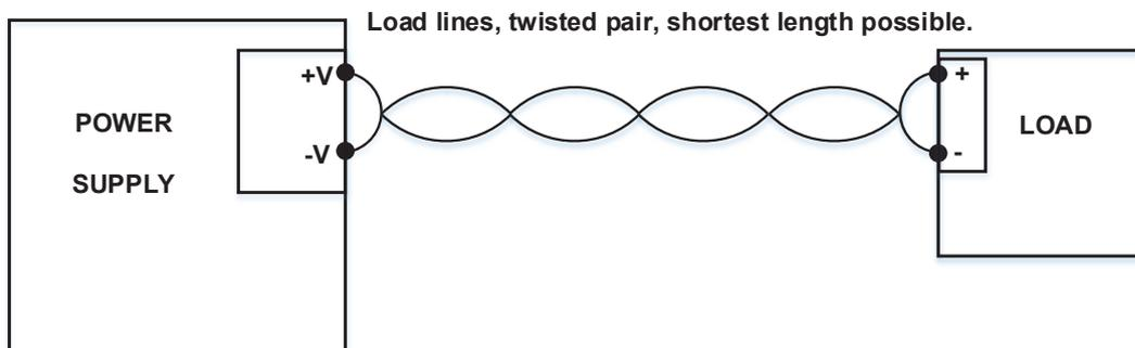
Figure 2–1: Single Load Connection, Local Sensing
