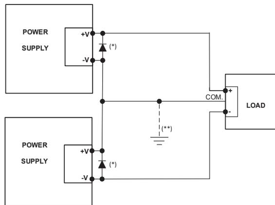
Figure 2–6: Series Connection for Positive/Negative Output Voltages
