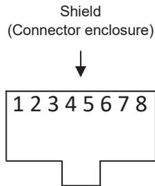
Figure 4–2: J3 Rear Panel RS485 OUT Connector Pinout
