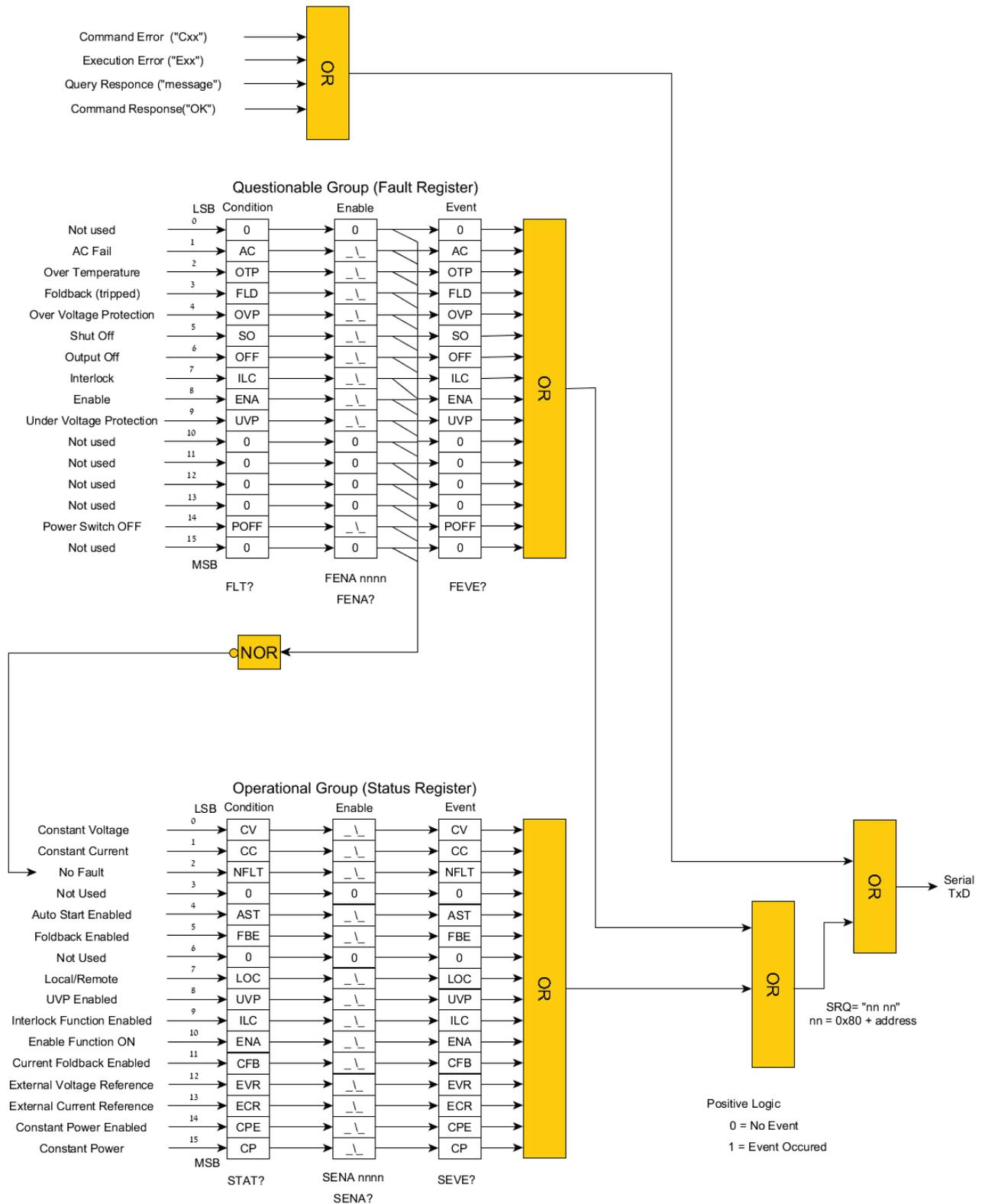
Figure 6–2: GEN Register Tree Diagram
