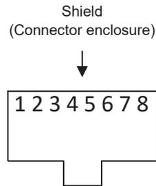
**Figure 4–1: J4 Rear Panel RS232/485 IN Connector Pinout**
