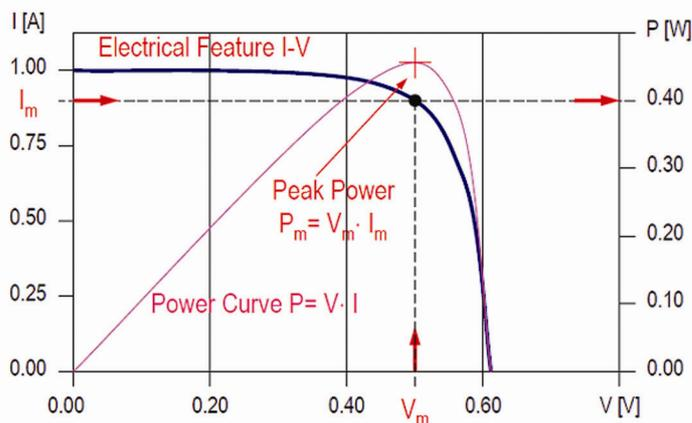
*Electrical Feature (I-V) and power curve for a single photovoltaic cell.*
