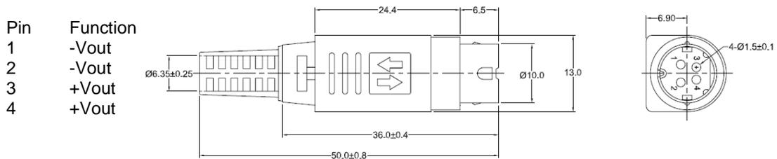
The DC output cable: 8C+1, UL2464, 16AWG, VW-1, 80°C, 300V
