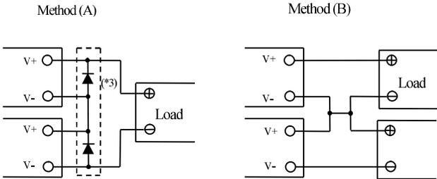
Note: In case of (A), please select a bypass diode (\*3) with maximum forward current rating more than output load current. And maximum reverse voltage must withstand each power supply output voltage. Never use when one of the unit not operate, which may lead damage.
