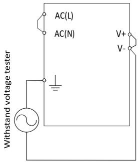
Note : In case of using external noise filter, capacitance between “Input and  $\perp$ ” might be increased. When testing withstand voltage between “Input and Output”, there is a possibility exceeding withstand voltage between “Output and  $\perp$ ” (1.5kVAC). Please check the voltage between “Output and  $\perp$ ”. If the voltage exceeding withstand voltage, please add external capacitor to “Output and  $\perp$ ”. It can decrease the voltage.
