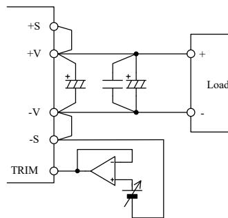
**Fig. 2-1 Output Voltage Adjustment
