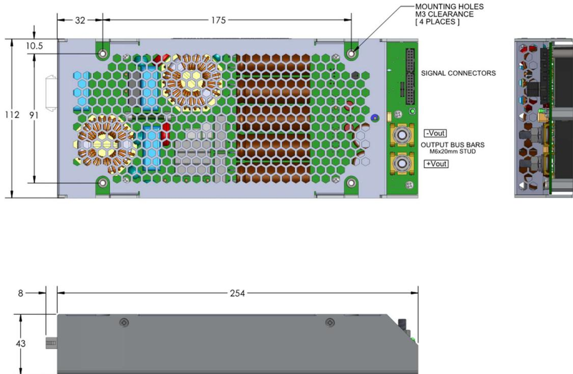
**Fig 28-1: Dimensions for Standard and /C chassis configurations**
