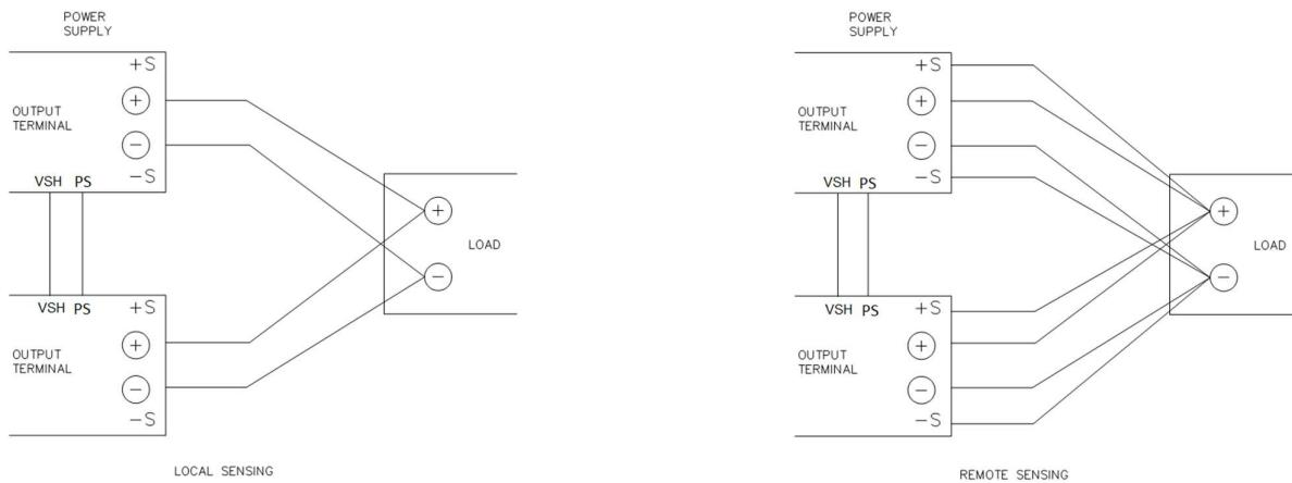
**Fig. 11-2 Parallel Operation**
