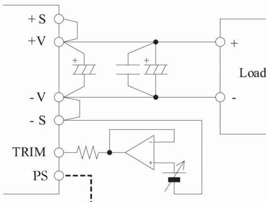
**Fig. 11-1 Output Voltage Adjustment by applying external voltage
