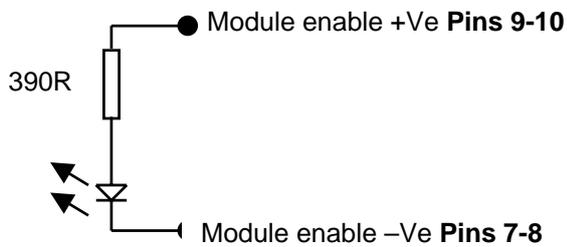
Internal to the module inhibit is a 390ohm 1/8W resistor and the diode of an opto-coupler.
