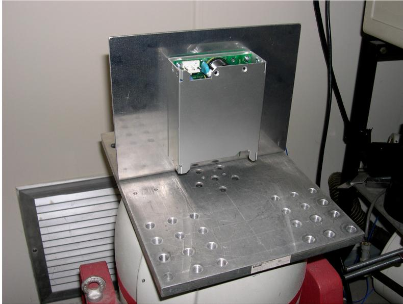
The unit was mounted onto a 3mm flat or right angle aluminium plate using the M3 customer fixings. The plate was in turn mounted to the vibration table. Mechanical inspection and Electrical testing was performed before the test. The following tests were performed :
