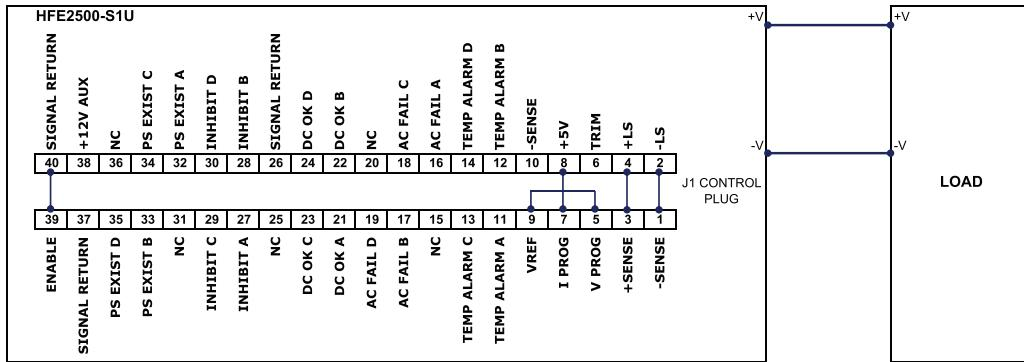
Fig 3.7 Output Voltage programming by PMBus
