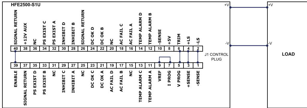
Fig 3.7.1 Output Current programming by PMBus
