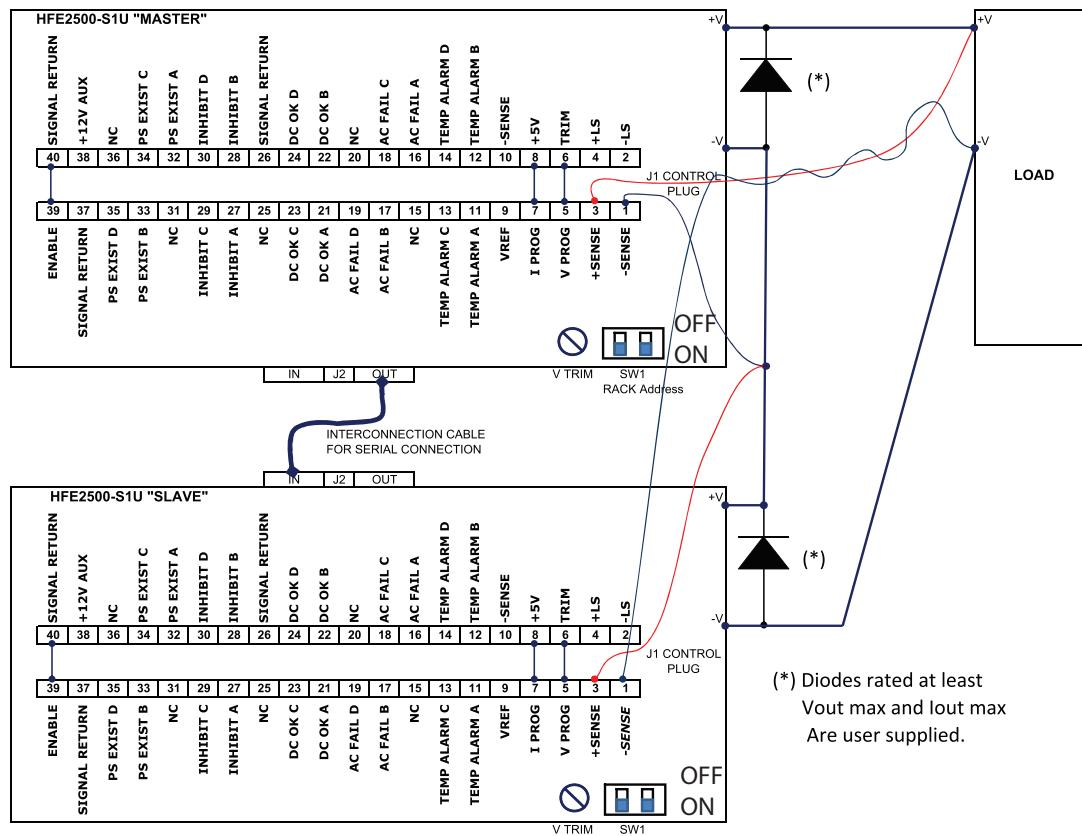
Fig 3.10 Serial connection diagram (remote sense).
