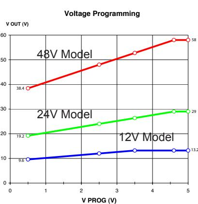
Fig 3.6 Output Voltage programming by External Voltage.
