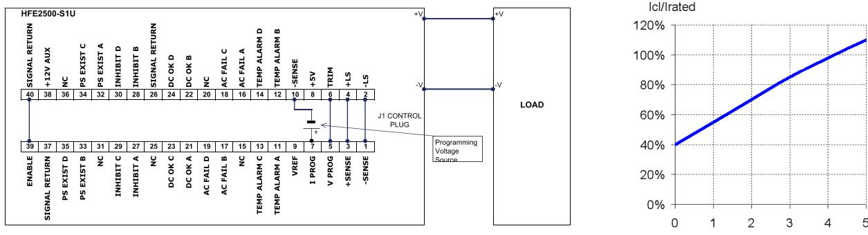
Fig 3.6.1 Output Current programming by External Voltage.
