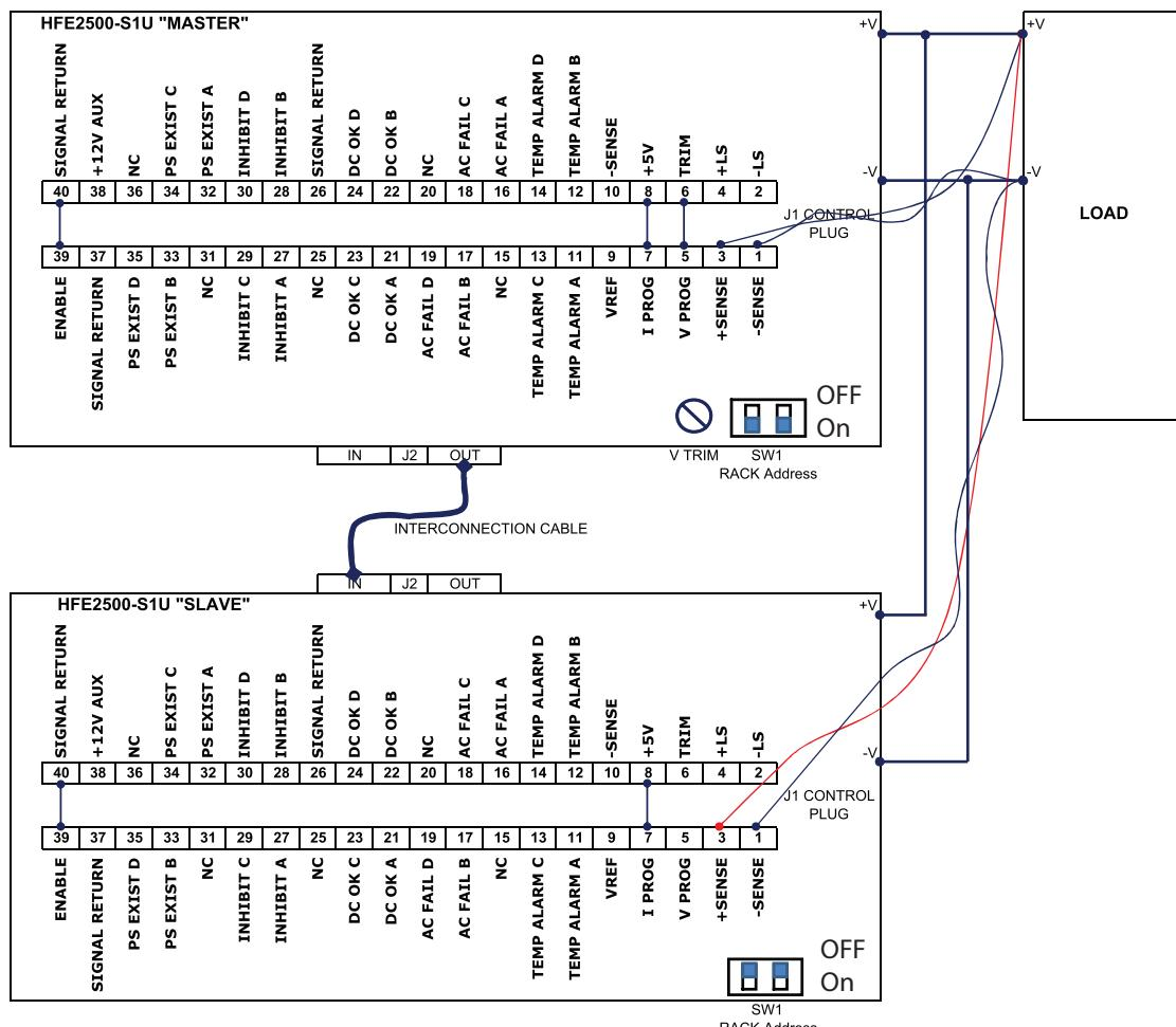
Fig 3.9 Racks parallel connection diagram.
