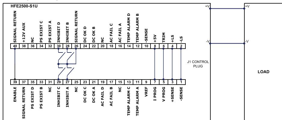
Fig 3.4 individual units On/Off diagram.
