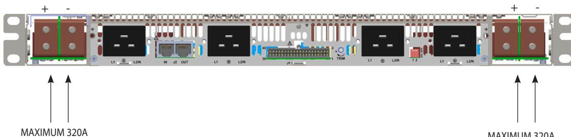
Fig 1.3a Output Bus-Bars.
