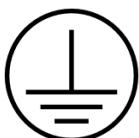
Protective conductor terminal. This is the terminal which is intended for connection to an external conductor for protection against electric shock in case of a fault.
