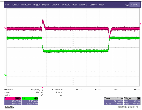
Load Transient Response. Load Step from 50% to 75% of Full Load with di/dt= 0.1A/uS. Ch. 2: Vo Ch. 4: Io
