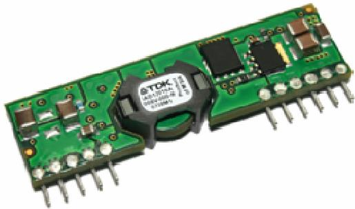
The iAD Series offers an 80W power module in the industry's standard SIP footprint. The iAD 12Vin series offers an ultra wide input voltage range of 6.0-14.0V. It is highly suitable for use in conjunction with 4:1 and 5:1 unregulated bus converters as well as with fully regulated 12Vout bus converters. The open-frame, compact design provides flexibility by performing local voltage conversion of a 12V bus. The single in-line package is well suited for almost any manufacturing environment.
