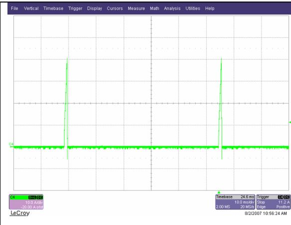
Typical Output Short Circuit Current
