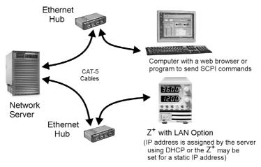
Fig.4-1: Server Network Connection Diagram
