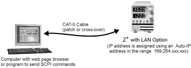
The computer is not connected to any other network
