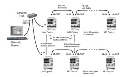
Fig.10-1: Configuring a Multi-drop System of Supplies
