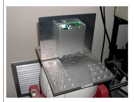
The unit was mounted onto a 3mm flat or right angle aluminium plate using the M3 customer fixings. The plate was in turn mounted to the vibration table. Mechanical inspection and Electrical testing was performed before the test. The following tests were performed:
