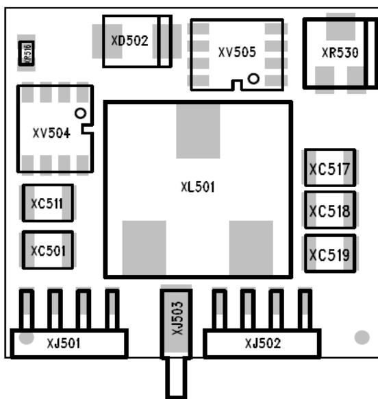
**SMA 3 channel 4 board (SMA 1 channel 2 5L, SMA 2 channel 3 xL, where x = 3, 5, T or F)**
