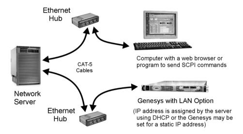
Figure 4. Server Network Connection Diagram
