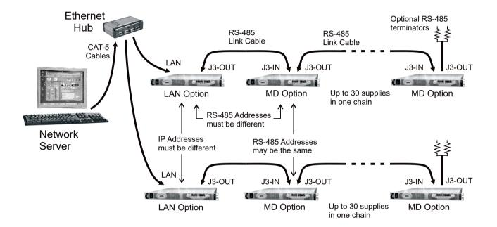
Figure 8. Configuring a Multi-drop System of Supplies
