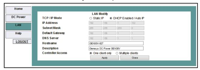
When the DHCP Enabled / Auto IP radio button is selected, only the following settings may be changed. The disabled settings (grayed) are set by the network's DHCP server.
