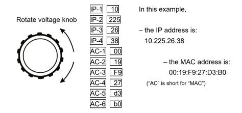
B. If the voltage knob is *not* changed for five seconds, the supply will revert to the normal voltage and current displays. If this happens, press and hold the FOLD button again.
