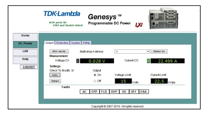
**Blink Identify:** When this button is clicked, the power supply front panel blinks and the rear panel LAN LED (Green) blinks. This function allows you to quickly identify which power supply is being communicated to in a rack of instruments. In a multi-drop chain, only the master LAN power supply will blink. You do <u>not</u> have to log in as 'admin' to use this control.
