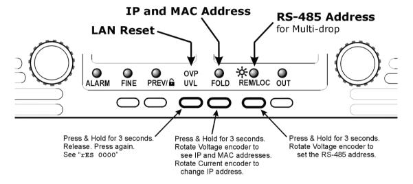
Figure 1. Front Panel LAN Features
