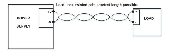
Figure 2-1: Single Load Connection, Local Sensing
