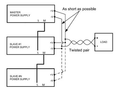
Figure 5-11: Parallel Connection with Local Sensing
