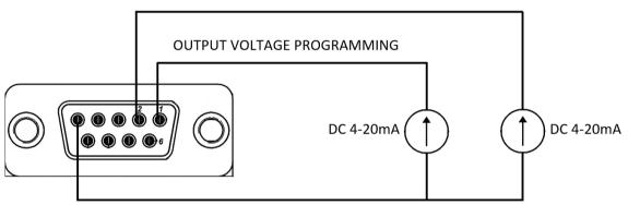
Figure 8-2: Isolated Analog Programming Wiring
