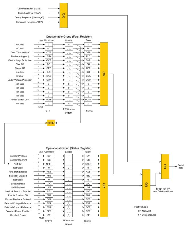
Figure 6-2: GEN Register Tree Diagram
