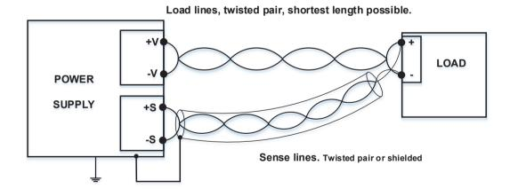
Figure 2-2: Remote Sensing, Single Load
