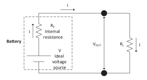
Figure 5-7: Internal Resistance Circuit
