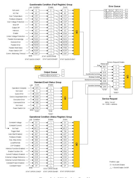
Figure 6–1: SCPI Register Tree Diagram
