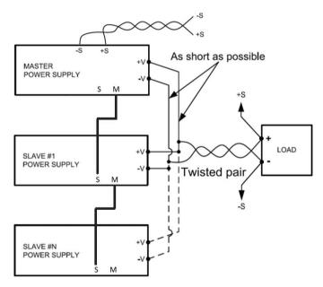
Figure 5-12: Parallel Connection with Remote Sensing
