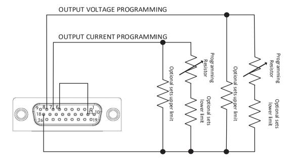
Figure 3–2: J1-Remote Resistor Programming Connection
