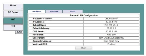
Figure 4-15: LAN - Configure Tab
