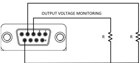
Figure 8–3: Isolated Analog Monitoring Wiring
