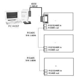
Figure 7–1: Point to Point Connection
