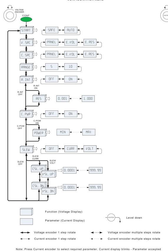
Figure 1–8: CONFIGURATION Menu Diagram
