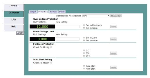
Figure 4-12: DC Power - Protection Tab
