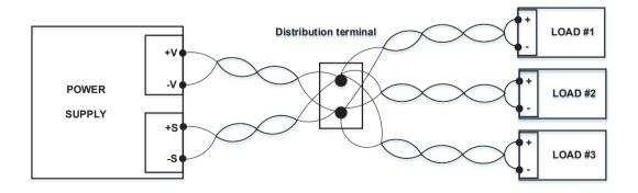
Figure 2-4: Multiple Loads Connection with Distribution Terminal
