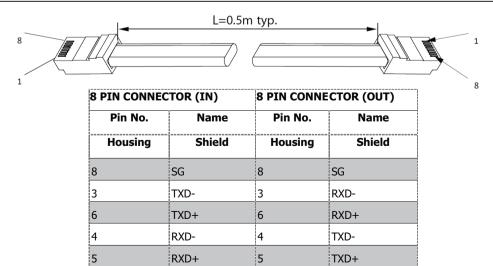
Table 4-2: Serial Link Cable with RJ-45 Shielded Connectors (P/N: GEN/RJ45)
