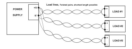
Figure 2-3: Multiple Loads Connection, Radial Distribution, Local Sense
