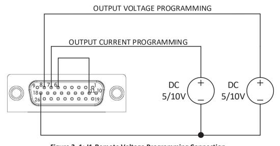
Figure 3–1: J1-Remote Voltage Programming Connection
