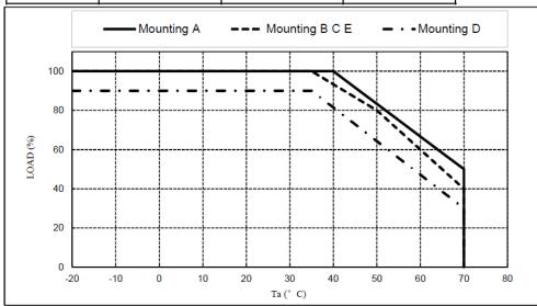
Condition B: Main output and standby mode power is derating according the following.
