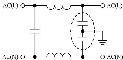
The example of noise filter circuit that may increasing capacitance value between "Input and  $\perp$  terminal". (Capacitance value dashed line is added.)
