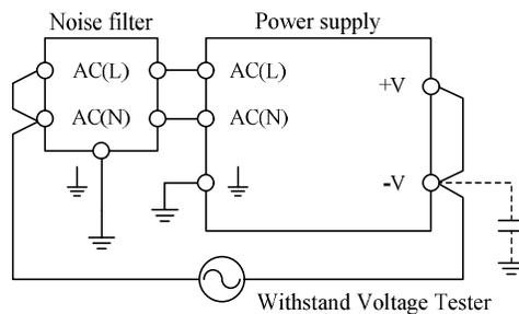
External capacitor adding point or short point. Even in the case of "+V and  $\perp$ ", there is a similar effect.
