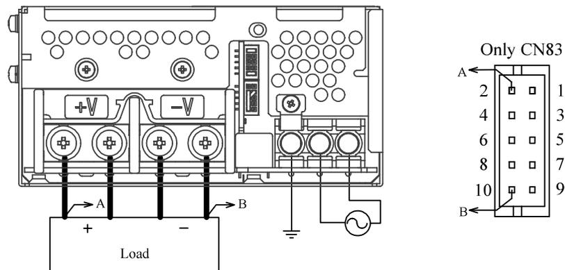
\*If remote sensing terminals are opened, the output will rise and shut down.
