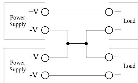
Note : Ensure that all units must be in operation. (Never use in condition that one of the units is not operated.)
