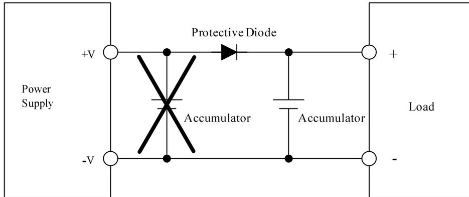
1. Adjust the output voltage higher by the value of forward voltage drop (VF) of the diode.
