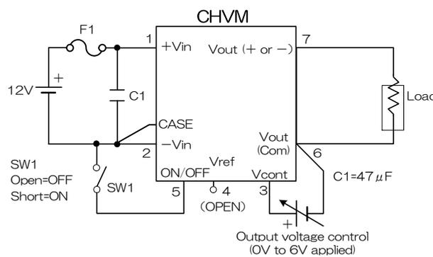
The CHVM series does not basically require additional parts, but add capacitor C1 to the input terminal if input impedance is high due to a long distance between the power supply and converter, an input line is thin, a filter is inserted on the input side, etc. When fitting a capacitor, try to add on the converter terminal side so as to reduce lead inductance.
