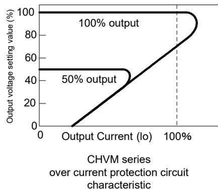
The overcurrent protection circuit shows a drooping characteristic. Ensure that the load to be used is at least with the minimum resistance specified for each series.
