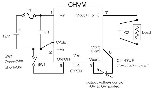
To reduce output noise even further, position C2 near the Load with the shortest input-output wiring while paying attention to creepage and spatial distances.
