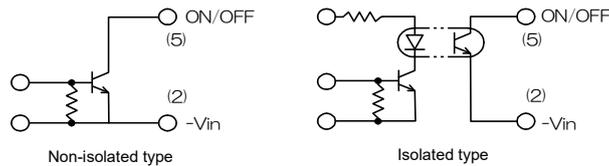
Ensure that there is no chattering to the ON/OFF terminal which affects output voltage. Output residual voltage is 0.5% or less when output is OFF under ON/OFF control (at the rated input-output).
