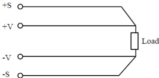
Ensure that the remote sense cables are twisted pairs.
