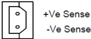
Remote sense can be used to compensate for the drop in voltage along the load cables or for the drop in voltage across blocking diodes. The voltage at the output terminals will be higher than that at the load by an amount equal to the voltage drop due to load lead resistance and/or blocking diodes if used. The maximum voltage at the terminals cannot exceed the maximum voltage specified for that module.
