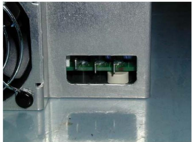
The AC input connection is situated adjacent to the cooling fan inlet as shown above. The faston tabs are tin plated 6.3 x 0.8mm at 9mm centres. Connection is made using insulated 6.35mm 'faston' connectors rated at 15amps each.
