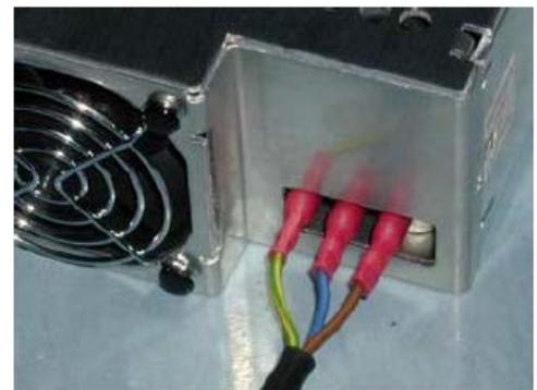
There is also available a screw terminal input version of Vega. This has a perspex safety cover and access to fit the screw terminals to the input is via 3 holes in the lid.
