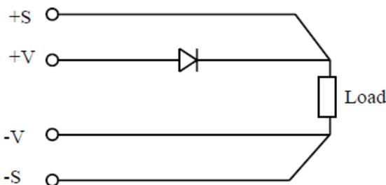
PCB power tracks and remote sense tracks should be kept away from each other as far as is possible.
