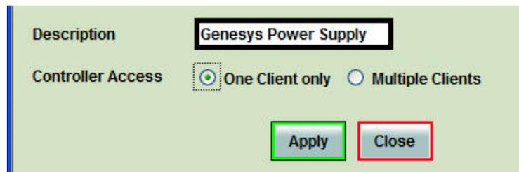
**NOTE:** *the performance of the Genesys™ LAN interface is impacted as more web pages, ports and sockets are opened at the same time. It is recommended no more than three be open at the same time.*
