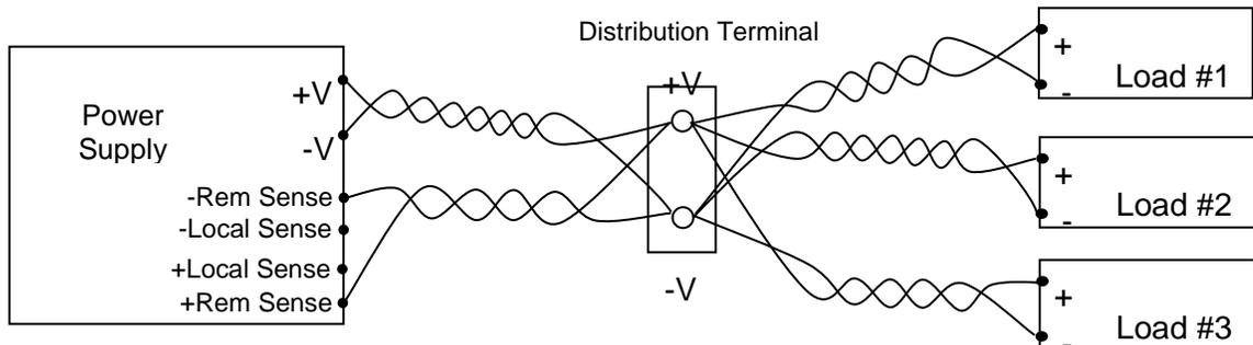
Figure 3-6. Multiple Loads Connected with Distribution Terminal, Remote Sensing
