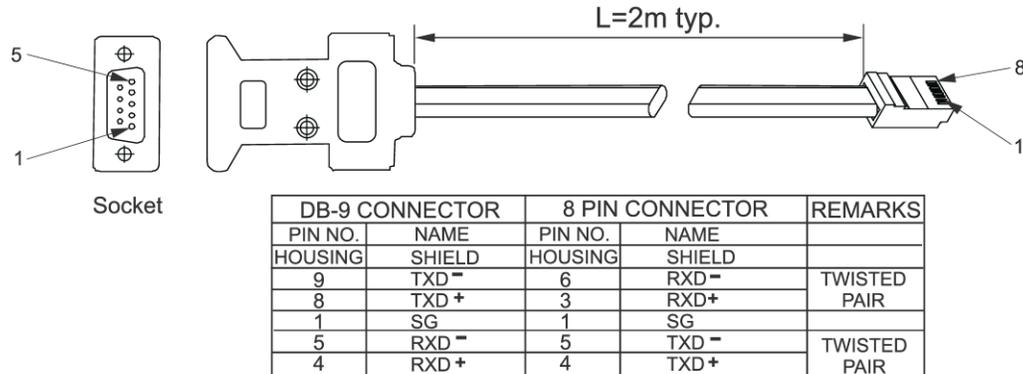
**Figure 8-4. RS-485 Cable with DB9 Connector (P/N: GEN/485-9)**
