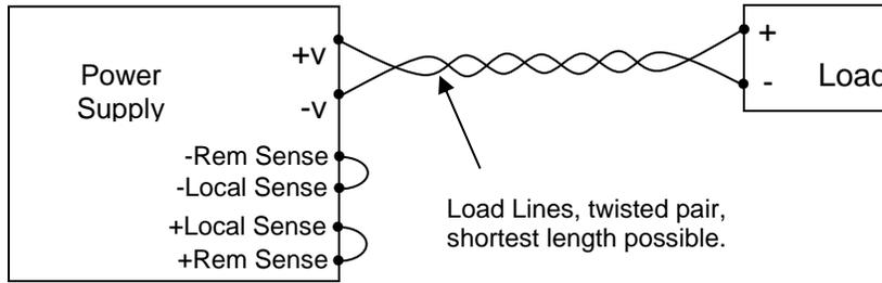
**Figure 3-3. Load Connections with Local Sensing**
