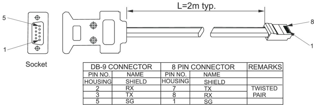
**Figure 8-3. RS-232 Cable with DB9 Connector (P/N: GEN/232-9)**
