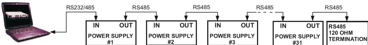
**Figure 8-5. Multiple Power Supply RS-232/RS-485 Daisy Chain**
