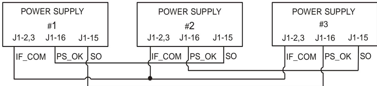
Figure 6-4. Shut-Off Daisy-Chain Connection
