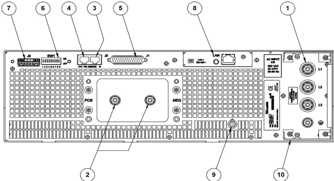
**Figure 4-2. Rear Panel Connections and Switches**
