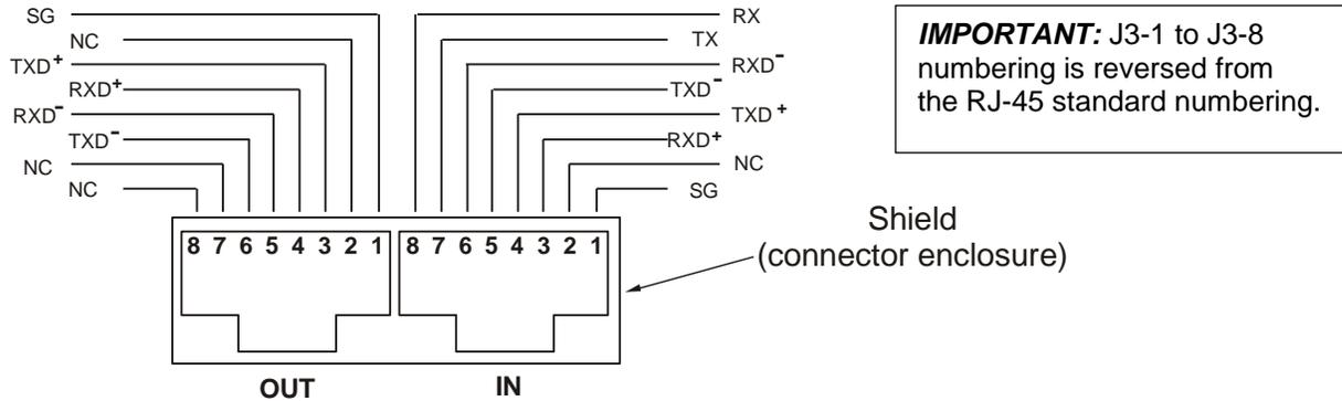
**Figure 8-1. RS-232/RS-485 J3 IN/OUT Connector Pin Out**
