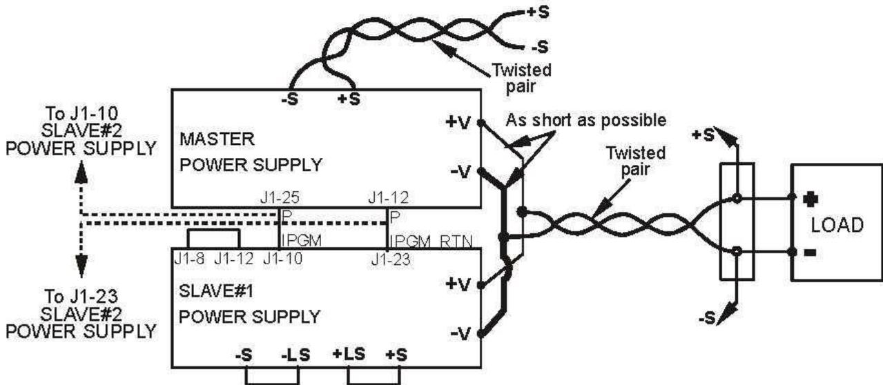
Figure 6-6. Parallel Supply Connections with Remote Sense
