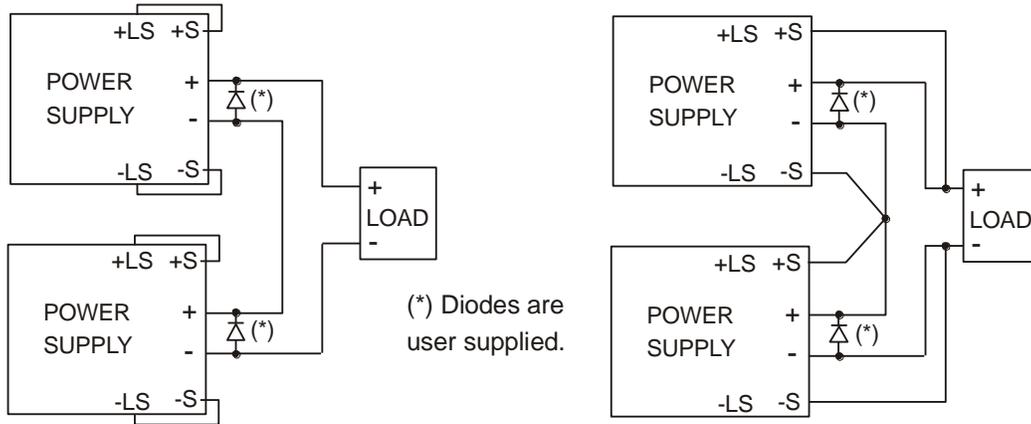
Figure 6-1. Series connection, Local sensing
