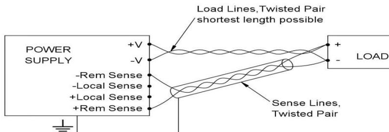
**Figure 3-4. Remote Sensing with Single Load**
