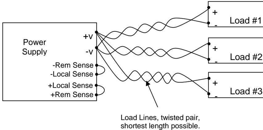
Figure 3-5. Multiple Loads Connection, Radial Distribution, Local Sense
