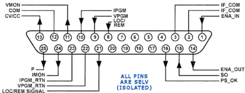
Figure 4-4. J1 Connector Pin Signals
