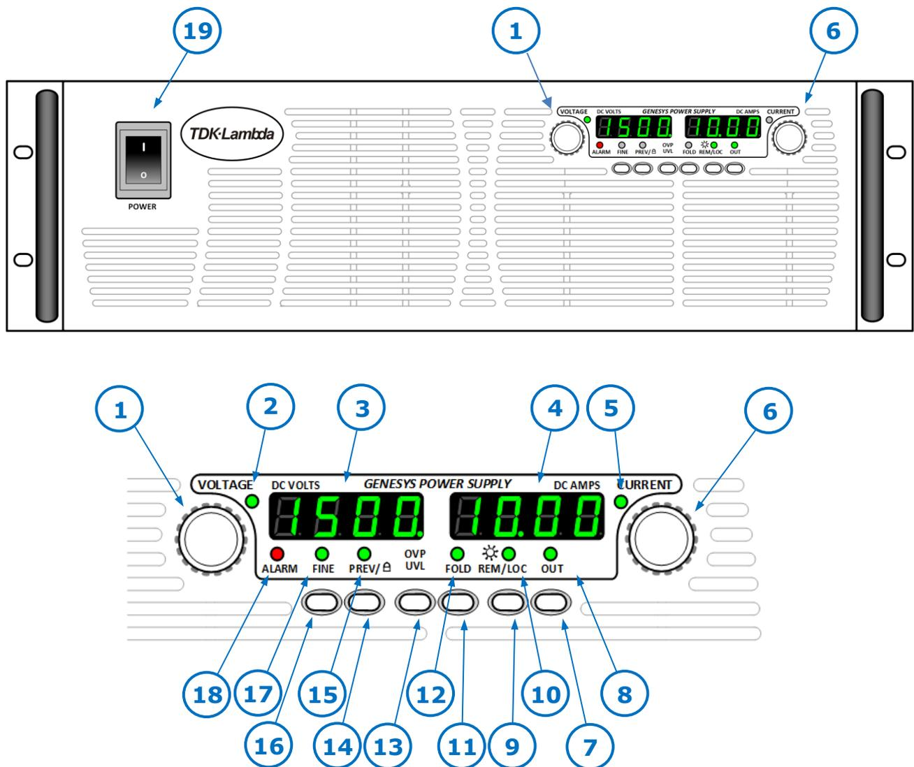
Figure 4-1. Front Panel Controls and Indicators
