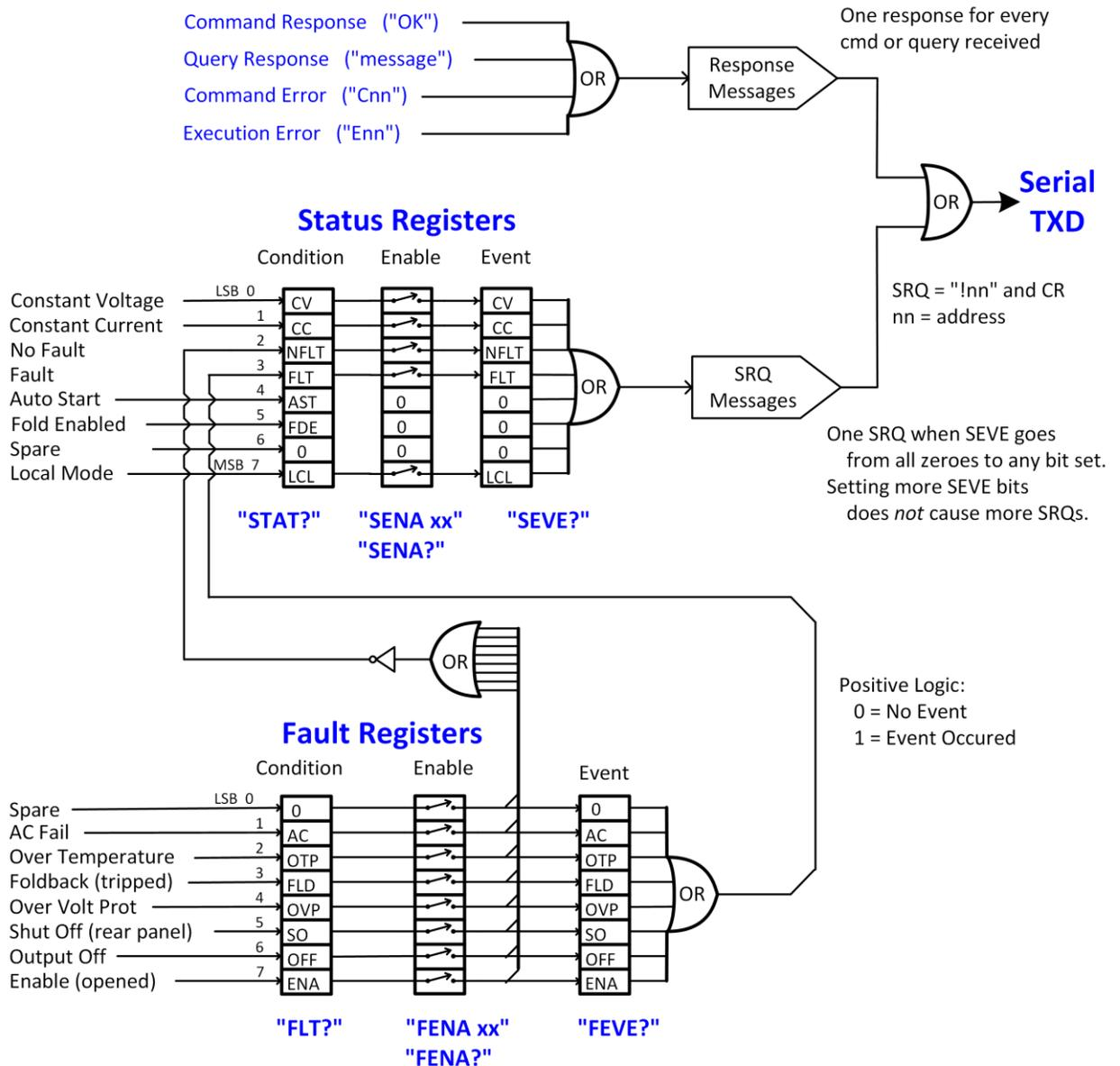
Figure 8-7. Status and Error Registers Diagram
